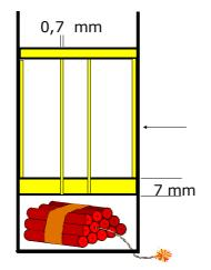
This is a smoke grenade. Smoke grenades are launched by putting them into a mortar, that is a tube with a driving charge at the bottom. The grenade is ejected by ignitiating the charge. Until a few years ago the grenades had to be made of metal. This meant cutting, polishing, soldering, etc., in other words a lot of metal work. With PHB you simply mold.
