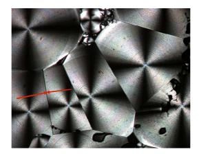
If you look carefully at the picutre you can discover tiny fissures between the crystals. This is a consequence of the different densities of the melt and the crystals. A close look at this picture explains what all science papers on PHB
