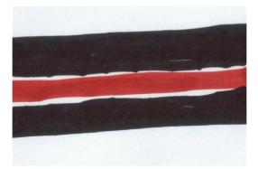
When one embeds fibers into the melt of PHB then the PHB matrix recedes from the hydrophilic fibers. Thus the fibers are free to move. It is possible to tear out small fibers with tweezers.
