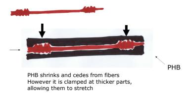
Here you see a slightly exaggerated picture of such a natural fibers composite to show the principle. The fiber still is free to move, but the movement is stopped at the thicker parts by pure mechanical means. There the hard crystal engulf the fibers like clamps.
