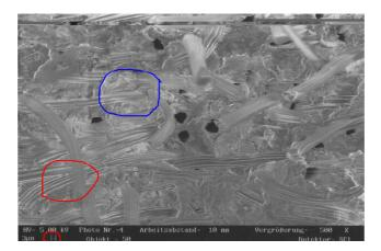
With long fibers the situation is different. At points where the leaves were attached before harvesting the fibers the fibers are thicker. The diameter increase only slightly, but exceeds the voids around the fibers. Such a situation is seen at the place encircled in blue.
