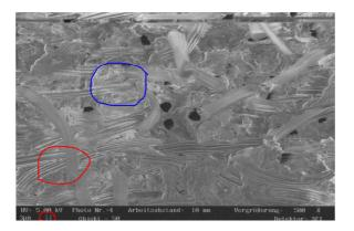
The picture shows the surface of a natural fiber composite. The bar at the left at the bottom (red) represents 3  $\mu$ . If you compare this bar with the imprints of the fibers, best seen a left (red) you easily can see that structures of well below one  $\mu$  are clearly displayed.
